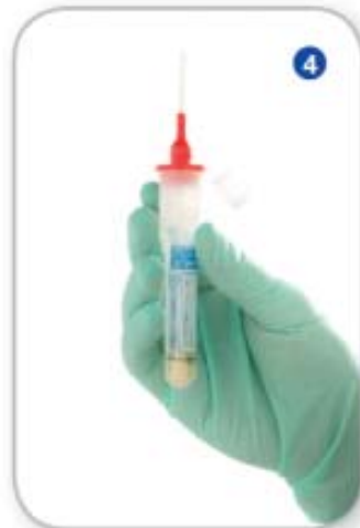
4. The media passes through the SWAB to enhance the release of bacteria into the broth
